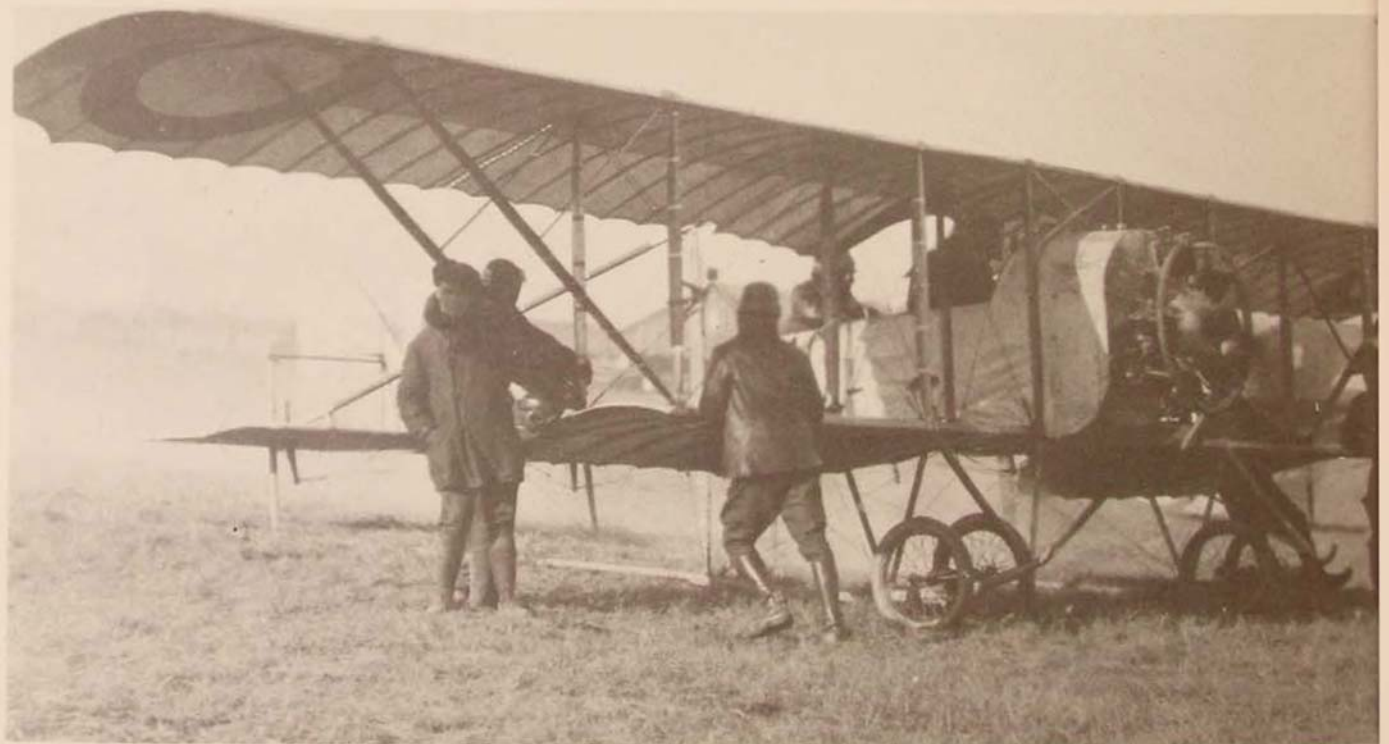
The Curtiss JN-4D "Jenny" (top), used as a primary flight trainer for American pilots, was a very forgiving aircraft. Advanced flight training in Europe normally meant flying battered aircraft that had been retired from combat service in favor of newer and better models. This French-built Caudron G-III (above) was used in 1915-16 as a reconnaissance aircraft and then brought back into service in 1918 to train American airmen.
